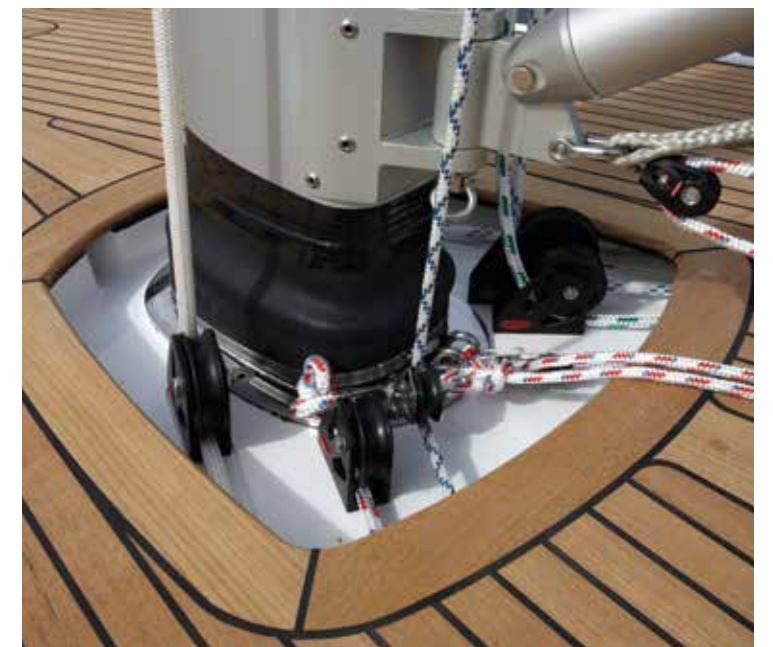
Optional vacuum applied teak on the coachroof. Split mainsheet passes below deck on both sides and is led back to the aftmost cockpit winches.
