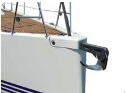
Standard GRP cowl with integrated anchor fitting
