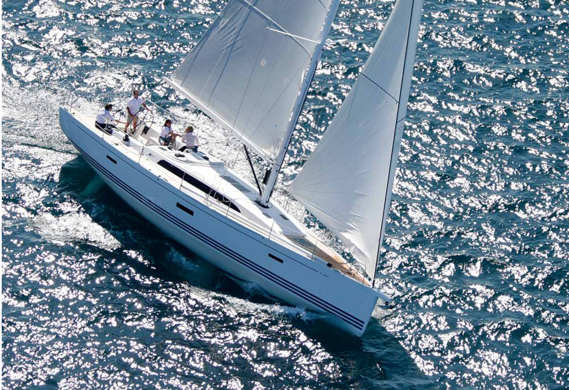
Left and centre: A custom-designed three-spreader alloy rig is supplied as standard, with a higher aspect carbon mast and boom available as an option
