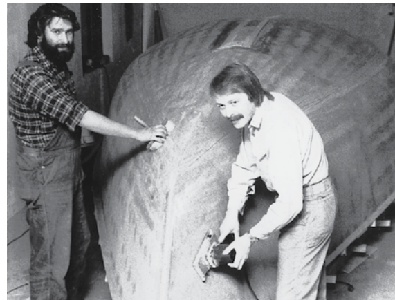
Niels Jeppesen and Birger Hansen building the hull plug for the first ever X-Yachts model, the One Design X-79. Almost 500 X-79s were built between its launch in 1979 and the mid-1990s
