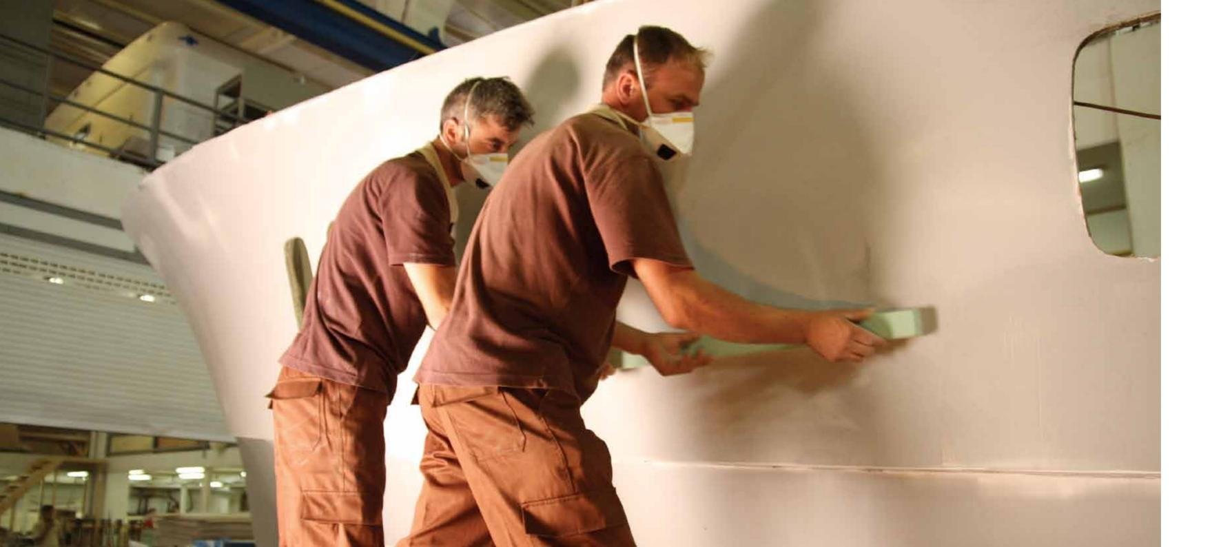
The mirror-like finish of the paintwork is the result of thousands of hours of personal attention by Zeelander craftsmen. Each Zeelander hull receives seven individual layers of paint and lacquer, with hand finishing between each layer by 6 craftsmen using long-boards. The process involves a clever blend of the automotive and aeronautic products to resist abrasion and ultra-violet damage. The result is then polished to create a luster that is unmatched in the yachting industry.
